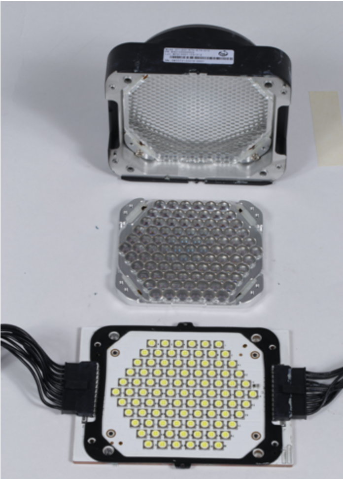
Opus X4's 1400 W LED array. Top: honeycomb and lens for a homogeneous surface. Centre: converging lenses for LED chips. Bottom: array diameter approx. 5 cm. Narrowest beam: 5.5°
